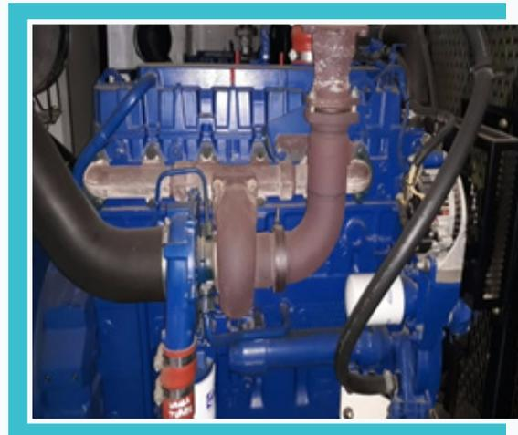
Gambar Sistem Turbocharger
