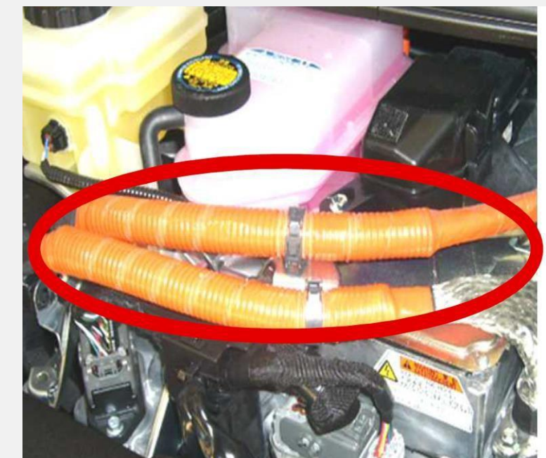
High Voltage Cable
