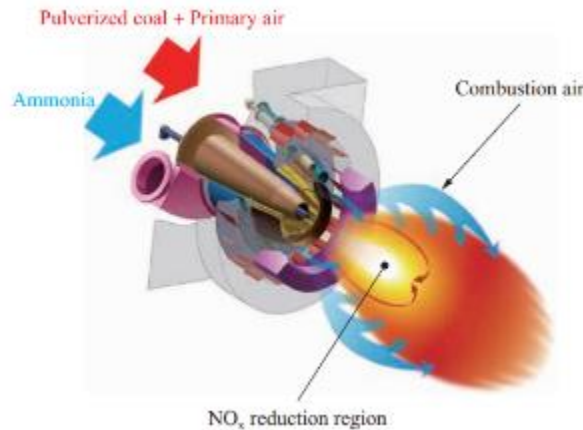
Schematic diagram of the modified burner to co-firing ammonia (ref. 1)
